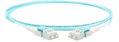
Uniboot Polarity Switchable Patch Cords feature high density, small form factor LC connectors mated to 2.0mm round duplex cable. They are used to connect switches or network devices in fiber networks directly or interconnect structured cabling systems in a fiber network. Polarity changes can be made in the field quickly, without the use of tools, to the correct fiber mapping polarity.
