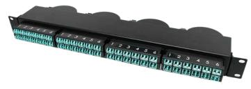
The static version Xtreme12<sup>™</sup> 1U panel is completely open for easy front and rear access. It is ideally suited for top of rack (TOR) applications. It can house up to 12 Xtreme12<sup>™</sup> modules for up to 144 ports. It can be ordered stand alone or with optional rear trunk cable manager.
