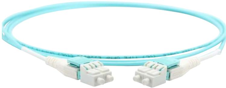
Uniboot Polarity Switchable Patch Cords feature high density, small form factor LC connectors mated to 2.0mm round duplex cable. They are used to connect switches or network devices in fiber networks directly or interconnect structured cabling systems in a fiber network. Polarity changes can be made in the field quickly, without the use of tools, to the correct fiber mapping polarity.
